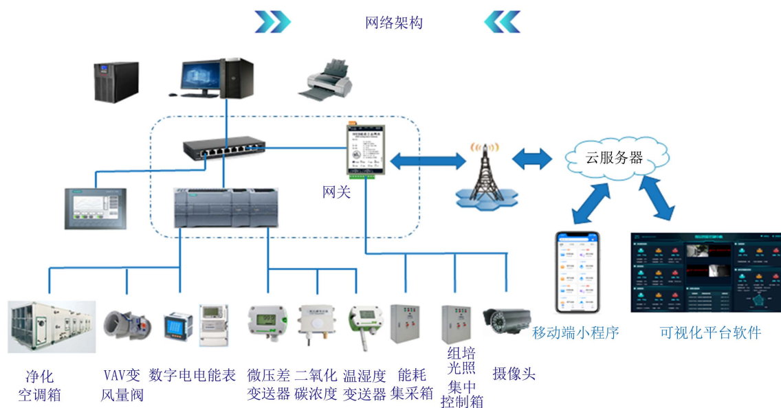
Figure 9. Network architecture of intelligent management platform for all-round tissue culture environment 图 9. 全方位组培环境智能管理平台网络架构
