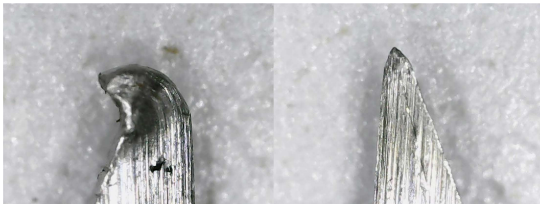
Figure 3. Knife-tip morphology after testing of metal and non-metallic material 图 3. 金属防刺层测试后刀头形貌(左)非金属防刺层测试后刀头形貌(右)
