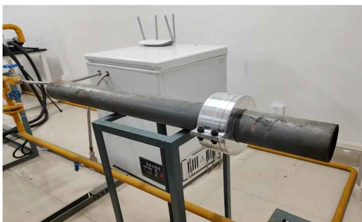
Figure 7. Excitation vibration descaling test bench
