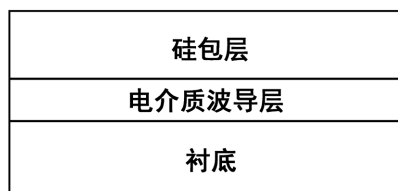
Figure 4. Optical waveguide model based on semiconductor cladding [44]
