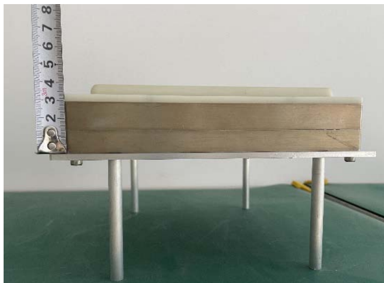
Figure 7. Photo of the L-Band low profile active phased array antenna 图 7. L 频段低剖面有源相控阵天线实物图
