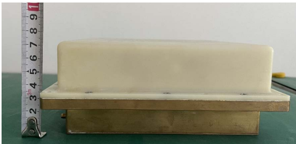
Figure 6. Photo of the L-Band brick type active phased array antenna with vertical extension
