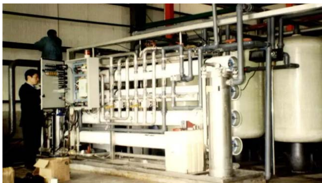
Figure 4. Nanofiltration membrane separation technology for industrial wastewater treatment 图4. 纳滤膜分离技术处理工业废水
