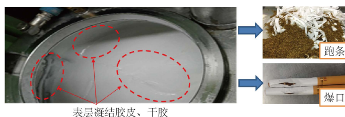
Figure 1. Glue collection, rubber skin, rubber block 图 1. 胶水集胶皮、胶块
