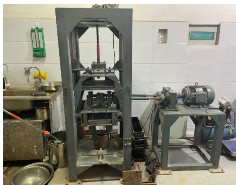
Figure 1. Surface vibration compactor
