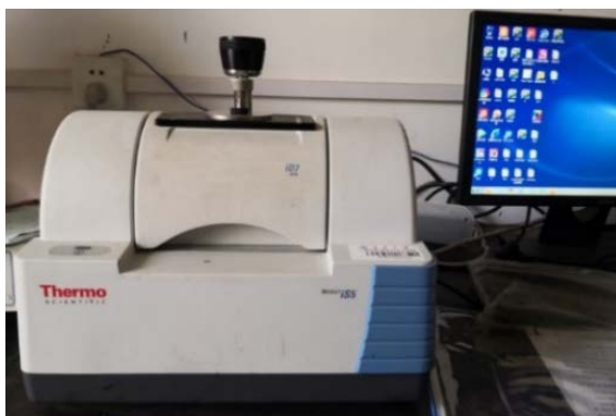
Figure 4. Nicolet iS-5 Fourier infrared spectrometer 图 4. Nicolet iS-5 型傅里叶红外光谱仪
