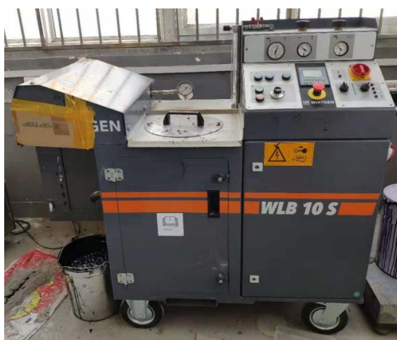
Figure 1. Asphalt foaming device 图 1. 沥青发泡装置
