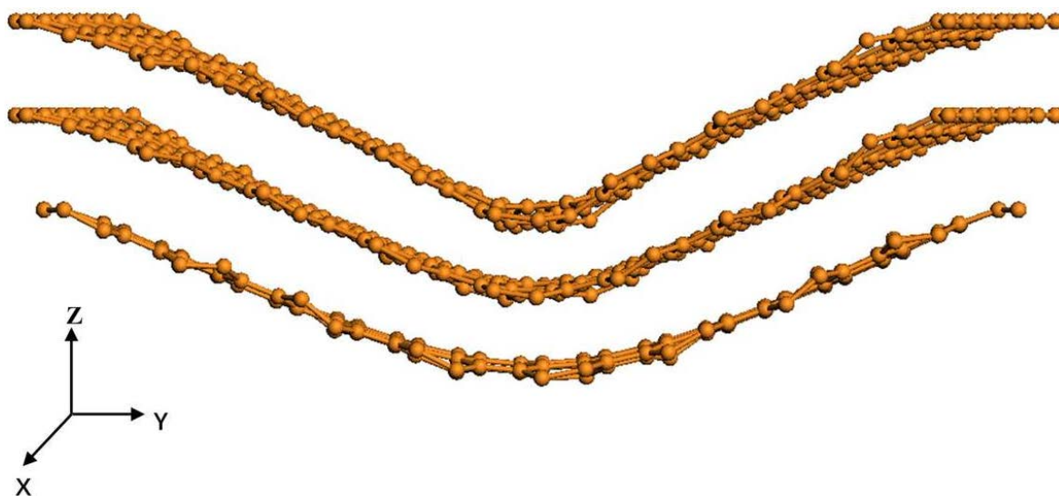
Figure 1. Schematic diagram of a three-layer graphene nanoribbon bent under compression, with the top two layers of the three-layer graphene layer rotated 15^\circ clockwise in the XY plane
