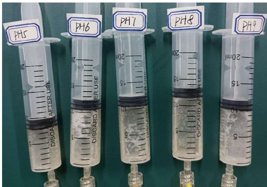
Figure 2. Comparison of calibration values of 20 mL cylinder piston at 5 min 图 2. 5 min 时 20 mL 针筒活塞刻度值比较图
