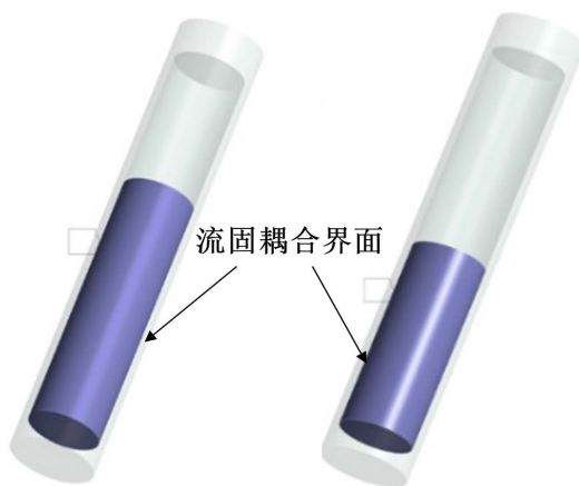
Figure 5. Definition of fluid-solid coupling interface in the accumulator barrel
