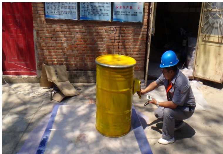
Figure 7. Carbon steel waste drum after cement solidification 图 7. 水泥固化后的碳钢废物桶
