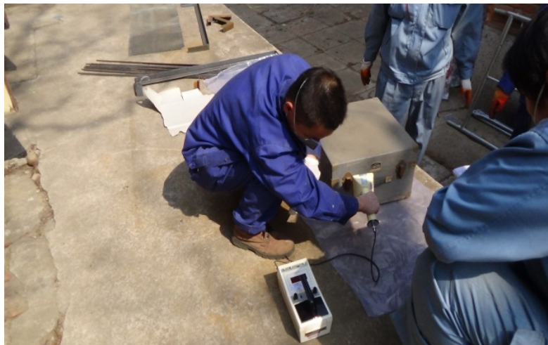
Figure 6. Radioactive measurement and classification of the disposed waste 图 6. 对清理出来的废物进行放射性测量分类
