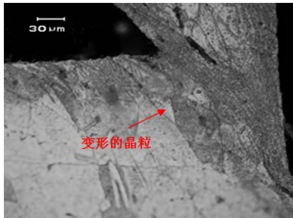
Figure 4. Metallographic picture of cutting root of deformed grain
