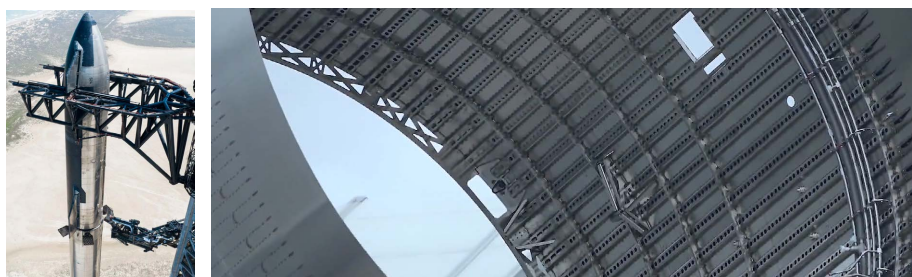
Figure 1. SpaceX's "supergrade-starship" welded with stainless steel
