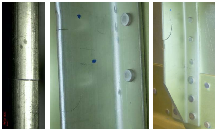
Figure 14. Hand riveted truss crack morphology of Al-Li alloy 图 14. 铝锂合金手工铆接桁裂纹形貌
