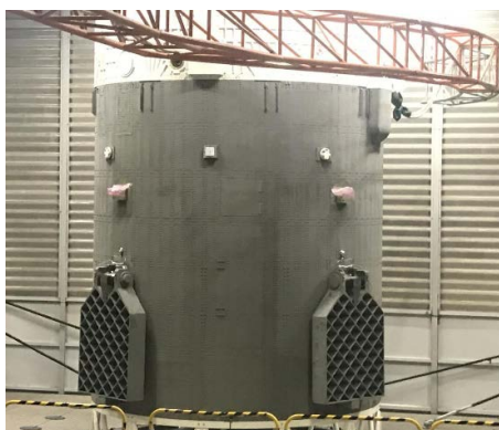
Figure 4. Expansion grid rudder structure of recyclable interstage segment 图 4. 可回收级间段展开式栅格舵结构
