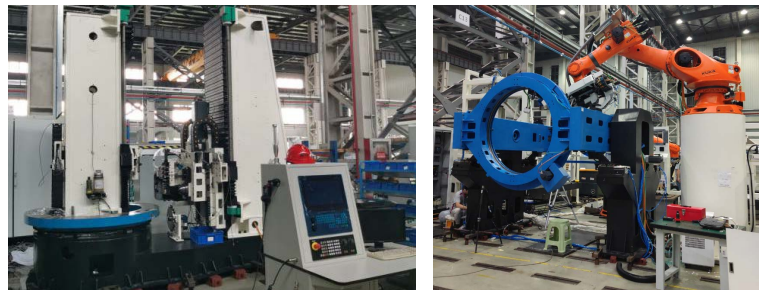
Figure 13. Automatic riveting technology of composite tank 图 13. 复合材料舱段自动铆接设备
