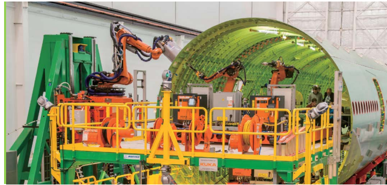
Figure 2. Automatic upright assembly system of fuselage 图 2. 机身自动直立装配系统
