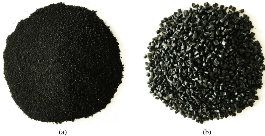
Figure 1. Two additives. (a) Waste rubber; (b) Waste plastics 图 1. 两种添加剂。(a) 废旧橡胶; (b) 废旧塑料
