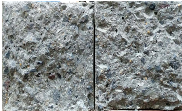
Figure 5. Splitting tensile typical failure surface 图 5. 劈裂抗拉典型破坏面
