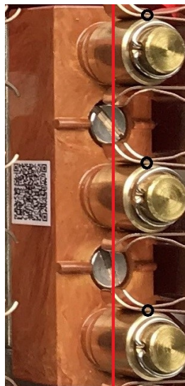
Figure 13. Contact position (black points) and outer horizontal coordinates of metal reeds (red line) 图 13. 接触点位置(黑色圆圈)与金属簧片外侧水平坐标(红色直线)
