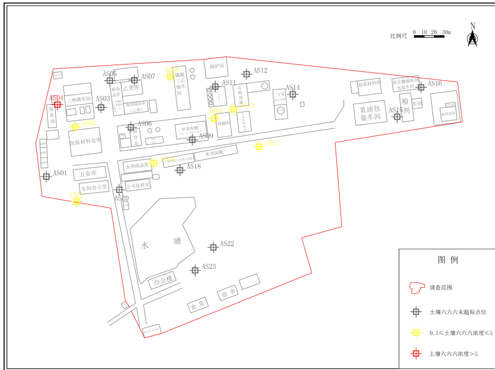
Figure 6. Schematic diagram of excess points of BHC in soil (mg/kg) 图 6. 土壤中六六六超标点位示意图(mg/kg)
