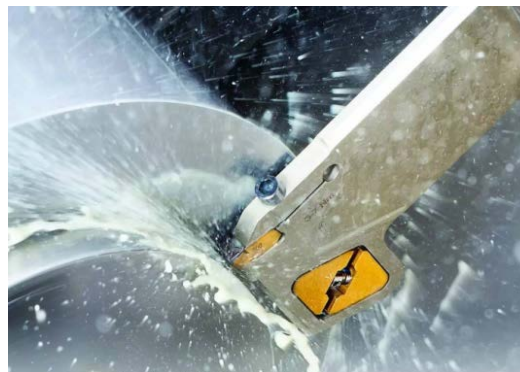
Figure 8. Damping module anti-vibration tool rod for Iskra circular grooving
