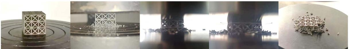
**Figure 3.** Compression process of original and artificially aged samples
