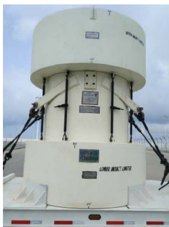
Figure 2. HDPE-HIC shielded transshipment container 图 2. HDPE-HIC 运输容器
